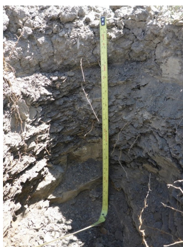
Figure 8. Soil Profile of a Shale Site.
