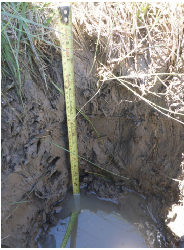
Figure 7. Soils profile of the Saline Subirrigated ecological site demonstrating the water table during the typical "high water table" period.
