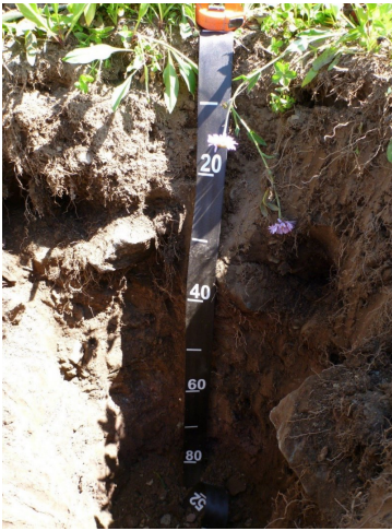
Figure 10. Close up view of a soil pit showing the high volume of fragments and skeletal nature of the soil.
