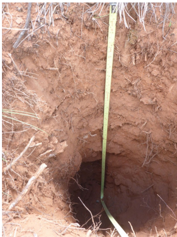
Figure 8. The chugwater formation provides a similar soil profile, with higher silts and the distinct red coloration.
