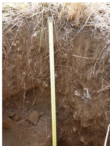
Figure 7. Soils pit, dug by hand, showing the deeper stony skeletal segment of a fine-loamy profile (upper soil layers 0-10 inches).
