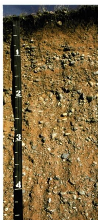
Figure 8. Soil Profile Image-Dix gravelly loam, Cheyenne County, NE. Depth is marked in feet.
