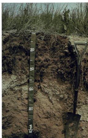
Figure 10.—Representative soil profile of Vonalee fine sandy loam. The argillic horizon is between depths of 15 centimeters (6 inches) and 48 centimeters (19 inches). The horizons below a depth of 48 centimeters (19 inches) contain calcium carbonate.
