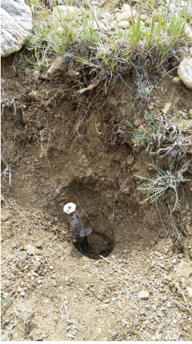
Figure 5. A typical Mion soil profile for the Slopes site. Note the gray shale fragments towards the bottom of the excavation, where developed soil grades into soft shale bedrock.
