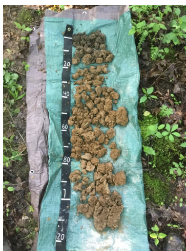
Figure 7. Del Rey Soil Series sampled on 05/29/20 in Dane County, Wisconsin.
