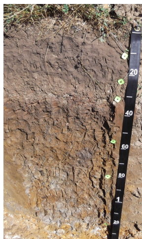
Figure 8. Soil profile of the Parsons series. Picture courtesy of Gene Campbell; scale is in centimeters.
