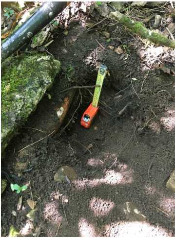
Figure 7. Galoo soil profile (soil depth is 7 inches)
