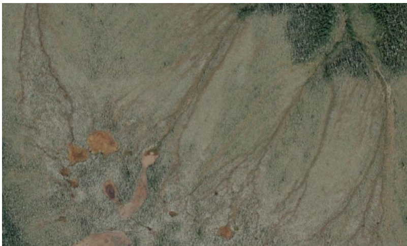
Figure 13. Pits and head cut gulleys on the toeslope and footslope of a hill caused by thermokarst in the area.
