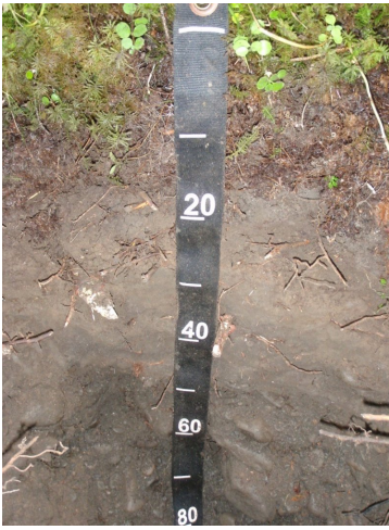
Figure 7. A typical soil profile associated with this site. These high flood plain soils are commonly coarse loamy over sandy or sandy-skeletal. Notice the sandy-skeletal alluvium at 50 cm depth.
