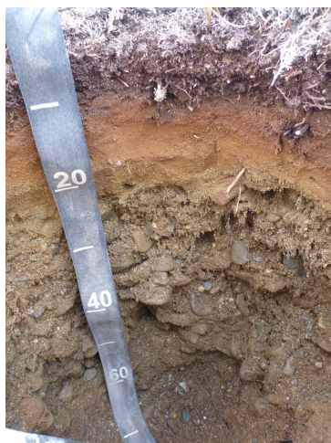
Figure 7. A typical soil profile associated with this site. Notice the layer of silty loess over the sandy and gravelly alluvium.
