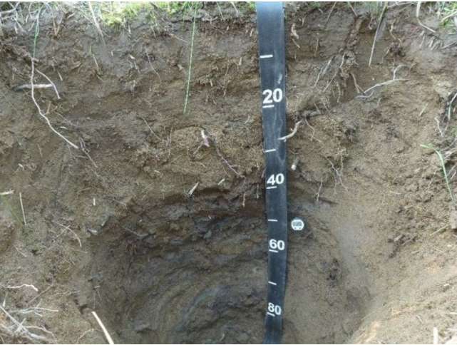
Figure 7. A typical soil profile on the low flood plain of montane streams in the area. The photo shows bands of silty and sandy horizons.
