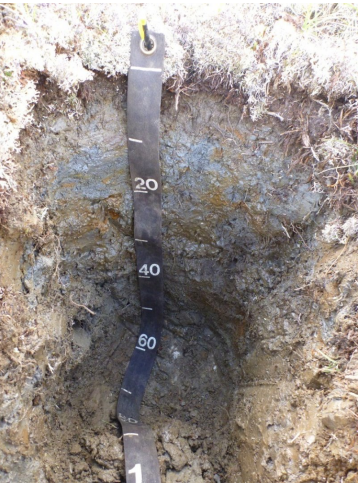
Figure 10. A typical soil profile associated with the non-sorted circle state.
