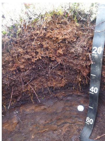
Figure 6. Typical soil profile associated with Sussaymin soil component.
