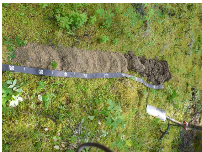
Figure 9. Teedrinjik soils have coarse loamy soil over sandy or sandy-skeletal material. The picture shows this change occurring at approximately 70 cm in the soil profile.
