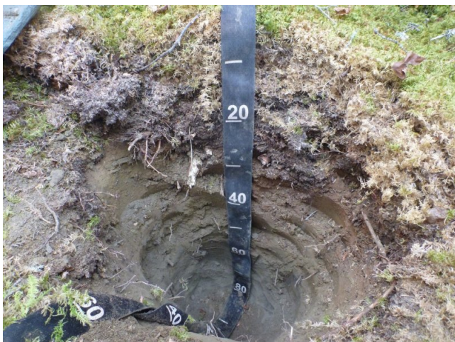
Figure 6. Typical soil profile associated with Folistic Haplorhels soil component. After fire, these soils often thaw resulting in Oxyaquic Haplocryept.
