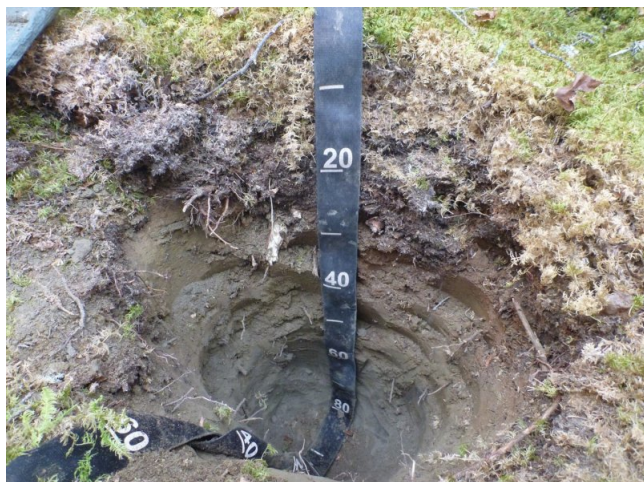
Figure 6. Typical soil profile associated with Folistic Haplorthels soil component. After fire, these soils often thaw resulting in Oxyaquic Haplocryept.
