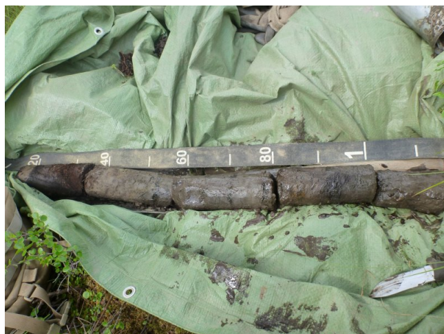
Figure 6. Typical soil profile of Ruptic Histoturbel soil component. Sample on tarp is a core from SIPRE auger.
